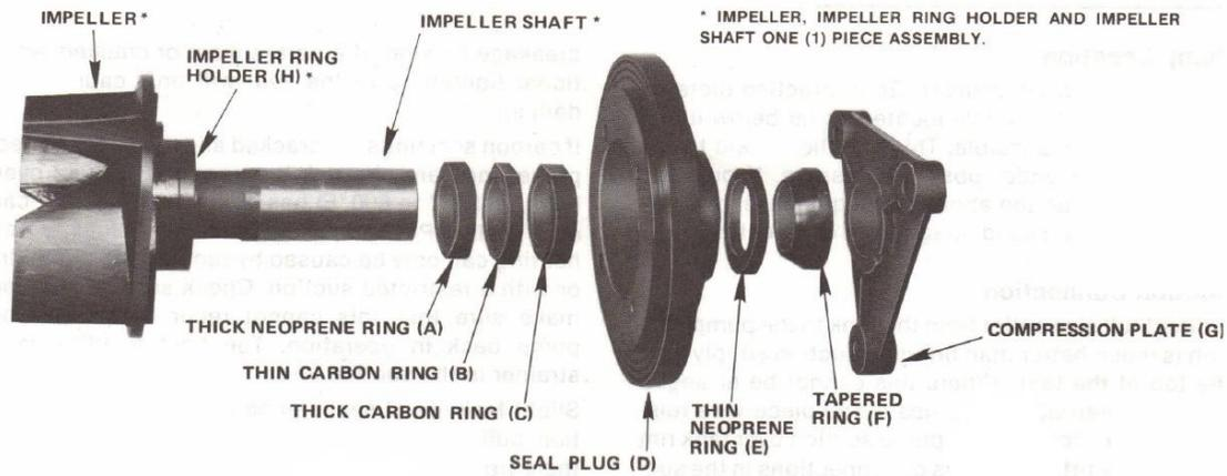
1. Install compression plate (G) onto the three studs on mount assembly. Install the rubber grommets, washers and nuts. **No tightening.**
